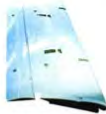
INBOARD FLAP (GFRP SKIN, NOMEX CORE)
